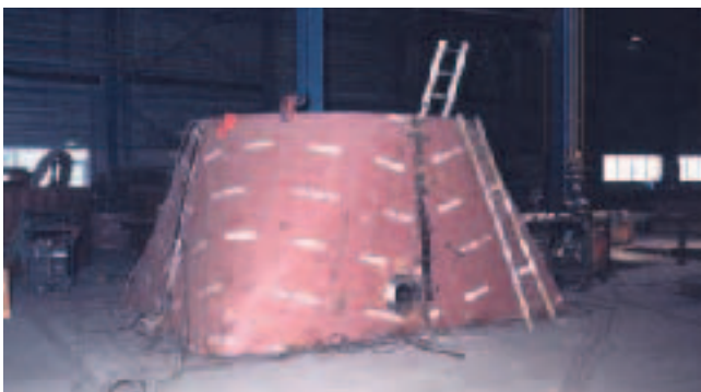
Figure 3. Crane pedestal part.
